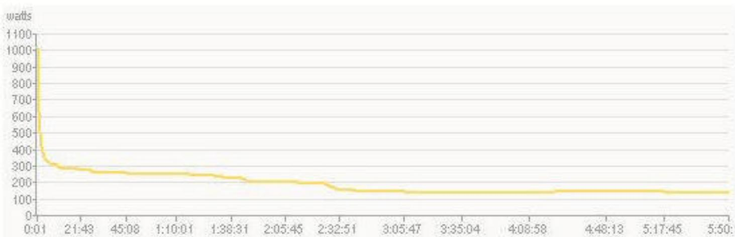
Figure 1. Sample of power-duration curve.
